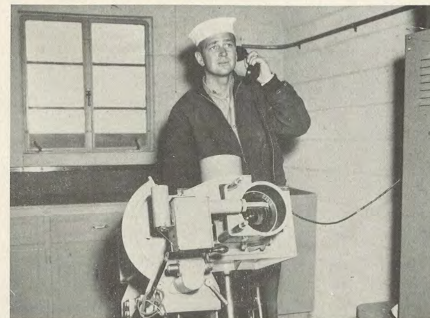
One of the more important WSPG optical instruments, the Bowen-Knapp ribbon frame camera, is manned by a sailor from the Naval Ordnance Missile Test Facility at WSPG. Bowen-Knapp cameras are used to record a pre-selected portion of a rocket's flight. (U. S. Army photo)
